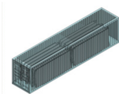
W-Tank® storage tank with 36 Salamanca plates, H=5m, D=25m and 2,534m 3 capacity transported in a 40-foot container.
